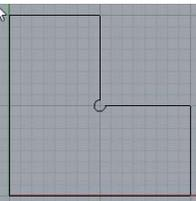
Redraw the part so you inside corners look like this. This will force Mach3 to cut into the corner. It also makes for clean breaks (bends).
