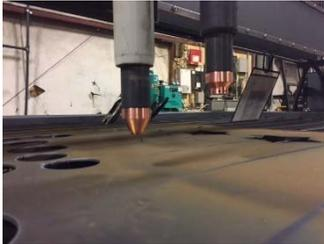
*The cutting torch and marking torch must be set up so that when the marker torch is in its down position, it is about 1" below the cutting torch. To do this, you simply move the torches up or down in the spring mount.*
