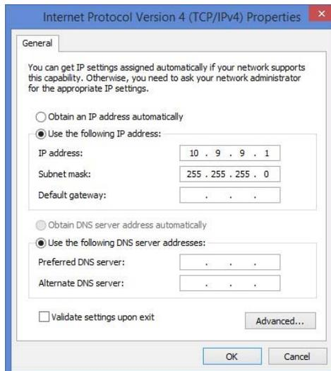
**NOTE: After making this change, connection to the internet will not be possible via the Cat5 Ethernet port. Use WiFi to connect to the internet.**
