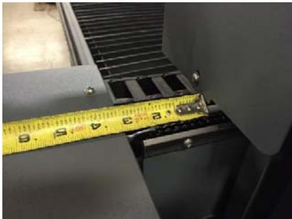
Repeat steps 2 – 9 on the Y axis. 40" works well for a 4x8 machine. 50" works well for 5x10 and 6x12. Restart Mach3 again after the Y axis has been set. You must restart Mach3 after each axis.
