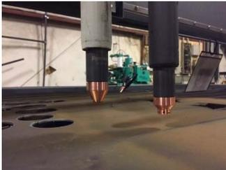
*This photo shows the marker torch in the down position. To raise and lower the marker torch, press the button called Marker Up/Down.*
