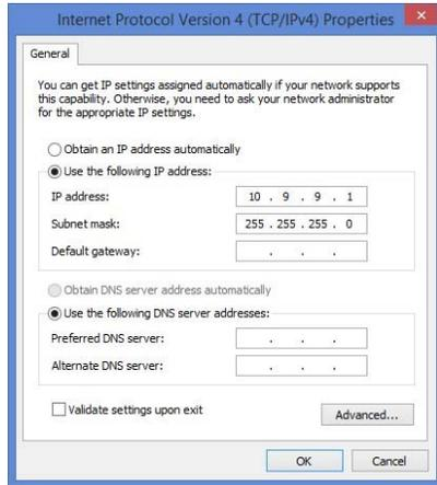
*has been modified, there will be one wired Ethernet port and one WiFi port. To get there, go to Windows Control Panel -> Network and Sharing Center. On the left click Change Adapter Settings. Right Click the Ethernet port and select Properties. Highlight Internet Protocol Version 4 and press Properties.*
